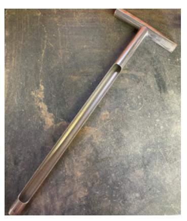
Figure 9.5 Soil probe.
