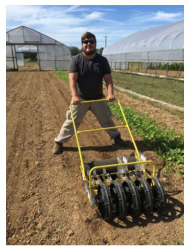
The ganged Jang JP-6 push seeder unit is heavier to maneuver, but the number of rows and spacing is customizable.
