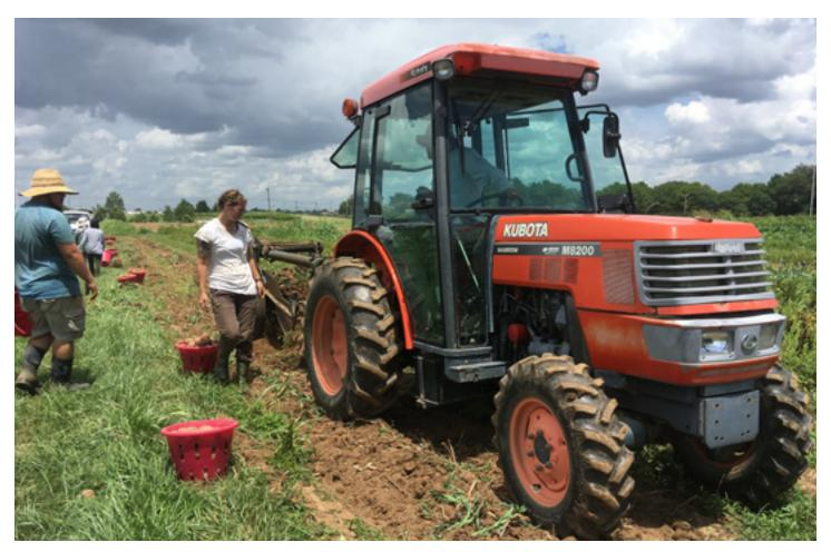
Potato harvest using the digger on the narrow Kubota M8200 tractor. Harvest buckets are spaced down the row.
