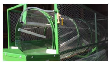
Figure 11.5 Barrel washer.
