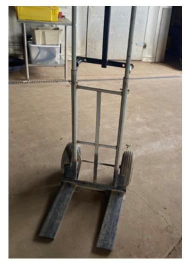
Figure 11.8 Custom hand truck with forks.
