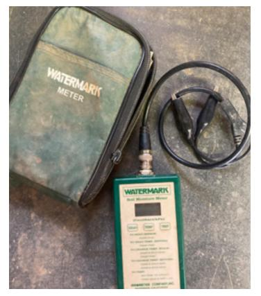
Figure 9.4 Watermark sensor meter.
