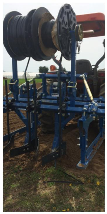
Figure 20. Custom Andros subsurface drip layer.
