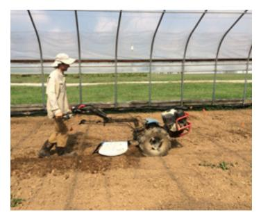
Figure 24. BCS rotary plow.
