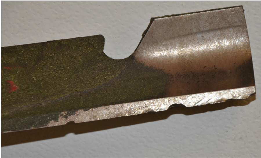
Figure 1. Dull mower blades increase mower fuel usage and potential for disease in grass plants.
