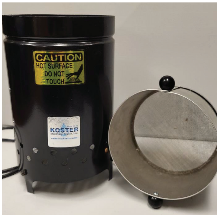
Figure 5. Koster tester available from farm supply companies, such as Nasco. Sample of fresh or fermented corn silage is added to the basket, weighed, and then placed on top of the Koster tester for drying. After sample is dry, the sample is reweighed and dry matter or moisture concentration is calculated. Photo: Nick Roy.
