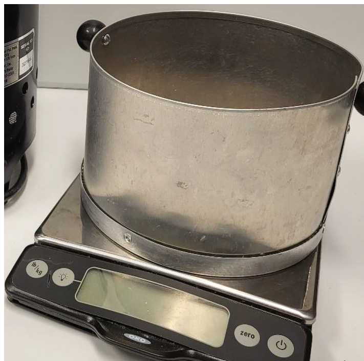
Figure 5. Koster tester available from farm supply companies, such as Nasco. Sample of fresh or fermented corn silage is added to the basket, weighed, and then placed on top of the Koster tester for drying. After sample is dry, the sample is reweighed and dry matter or moisture concentration is calculated. Photo: Nick Roy.
