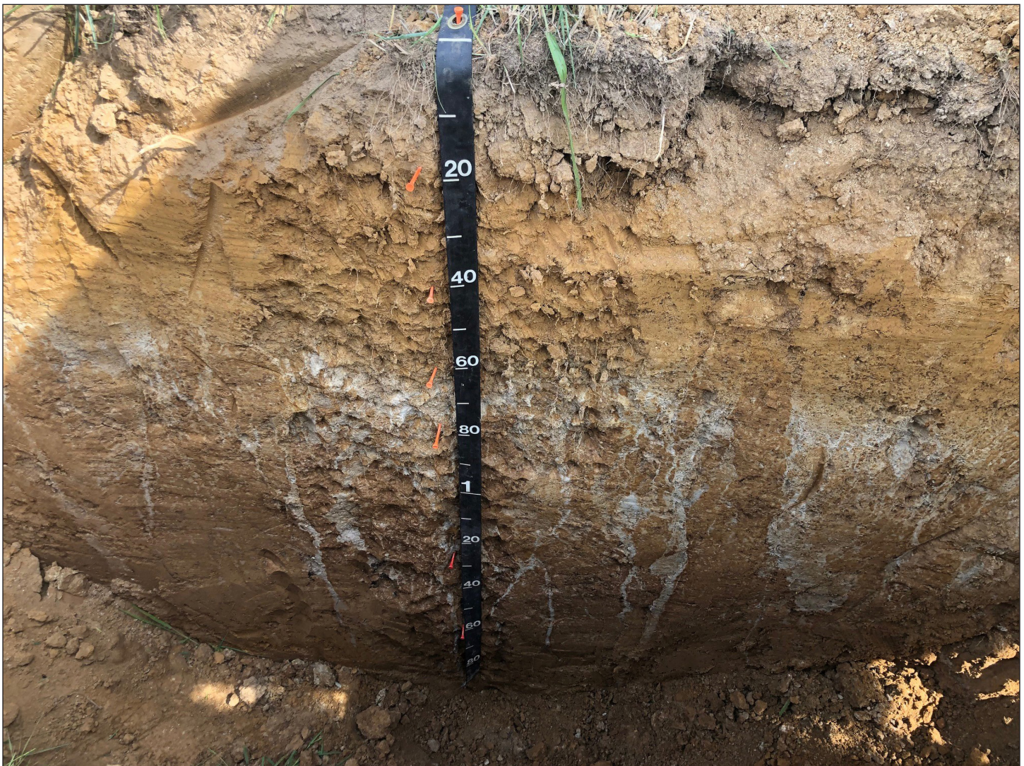
Figure 8. Soil profile of a fragipan beginning at 60 cm (24 inches) and extending to the bottom of the pit.
