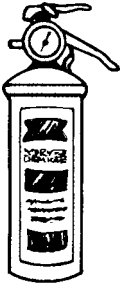
Figure 1-1 KEEP A FIRE EXTINGUISHER ON HAND IN THE TRACTOR SHED. MAKE SURE IT IS APPROVED FOR USE ON PETROLEUM FIRES.
