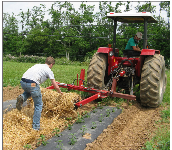
Figure 5. Round bale rolled out to small diameter with the offset bale unroller.
