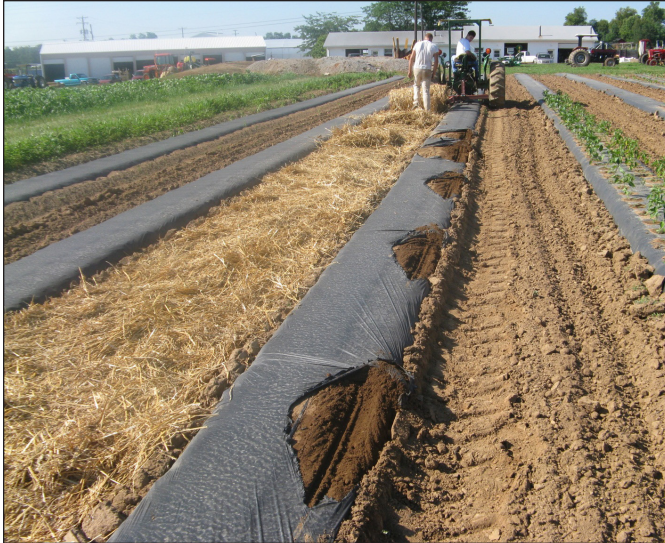
Figure 6. Damage to plastic mulch caused by the toolbar when using a fixed-length top link.
