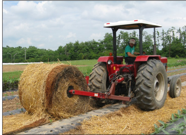
Figure 1. Offset bale unroller unrolling a round bale of straw between rows of plastic.
