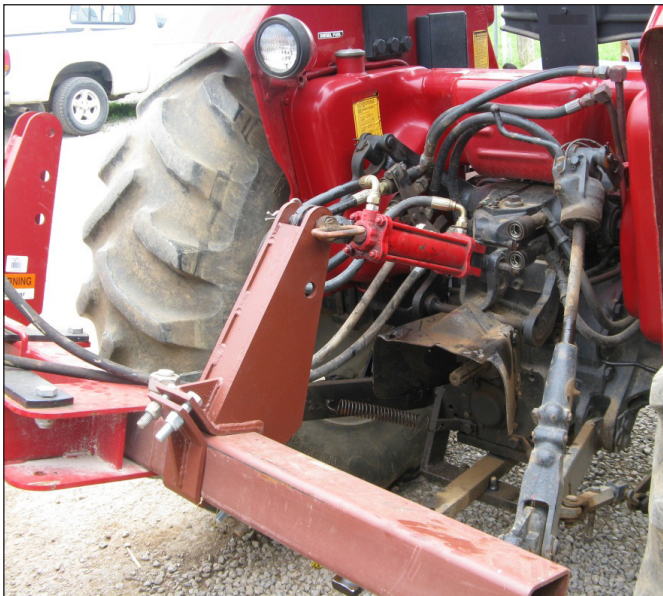
Figure 4. Hydraulic top link used with the offset bale unroller.
