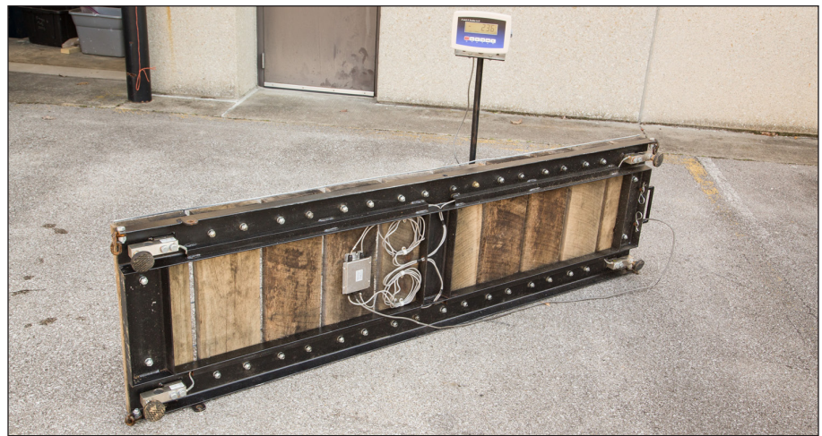
Figure 15. Location of junction box and wiring underneath the platform scale.
