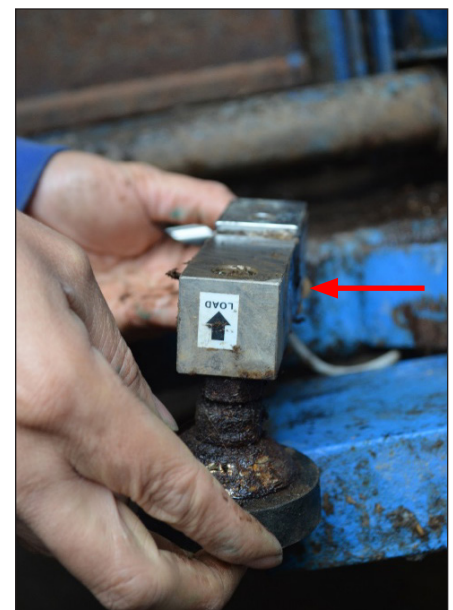
Figure 10. Arrow points away from feet of load cell. Spacer block is shown on top of load cell (red arrow).
