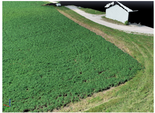
Figure 4. An isometric top view of a portion of a fully processed alfalfa field model flown on June 4, 2019, using Flight 1 parameters. Only part of the nearby barn is modeled as the flights only recorded one side of the building.
