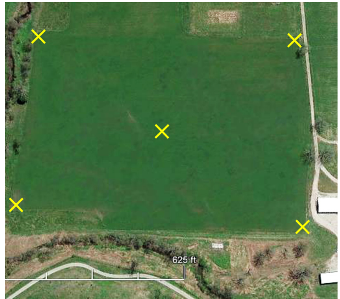
Figure 3. GCP best practices. Collect five to ten points per field distributed in a grid-like pattern as indicated by the Xs.
