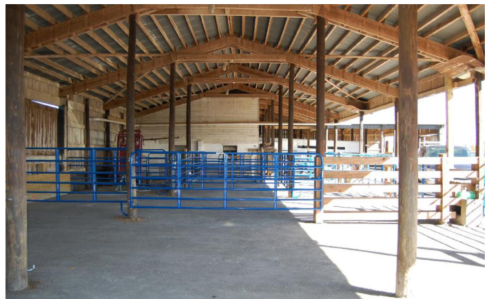
Figure 10. The flexible interior layout includes subdivided maternity and sick pens, along with an added handling facility (back left corner), to better utilize square footage.
