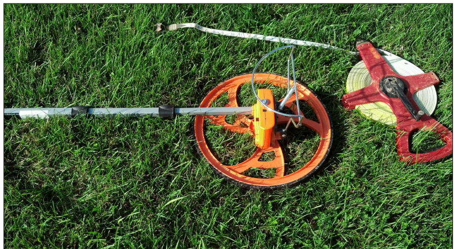
Figure 3. Common tools for measuring the area of the lawn: a walking wheel and a measuring tape.
