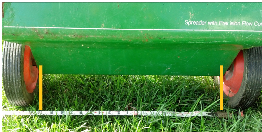
Figure 6. Measuring the effective width of spread for a drop spreader. The width is determined directly below the hopper, between the yellow lines.
