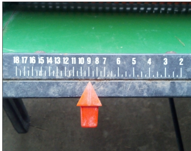
Figure 8. Choosing a middle setting for the spreader is a good starting point.
