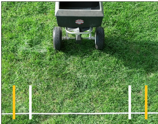
Figure 7. Measuring the effective width of spread for a rotary spreader. The total width (between the yellow lines) is multiplied by 0.75 as most of the fertilizer is thrown within 75 percent of the total width (between the white lines).
