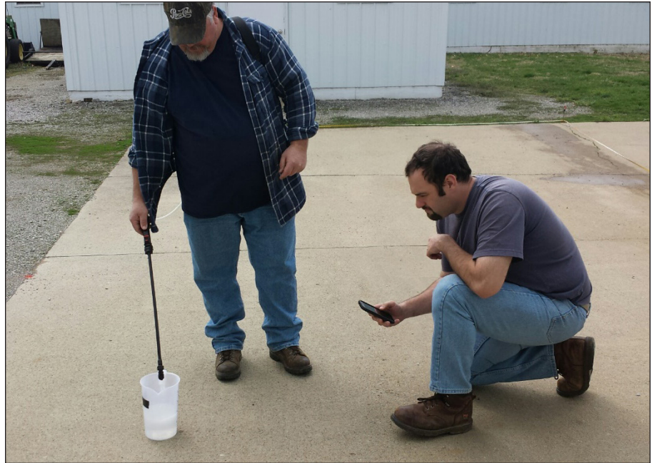
Figure 2. Spraying into the measuring container for the same length of time it took to spray the square.
