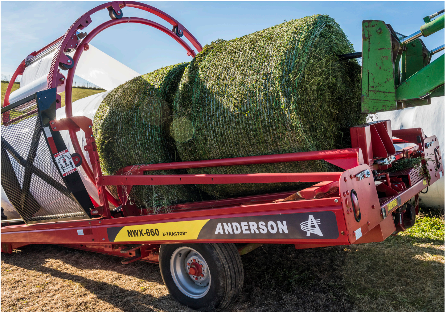
Making baleage with an inline implement is faster than an individual wrapper and uses less plastic.
