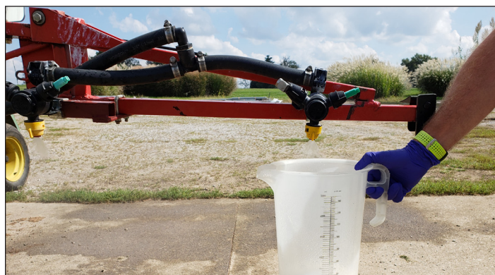
Figure 3. Collecting nozzle output for same length of time as it took to travel the pre-determined distance.
