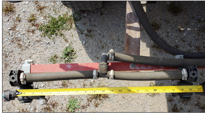
Figure 1. Measuring nozzle spacing in inches from the center of one nozzle to the center of the next nozzle.
