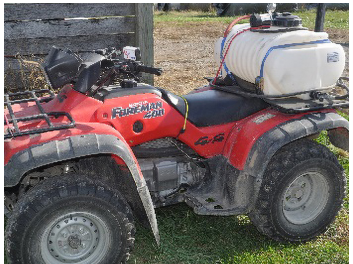
Figure 6. Inexpensive sprayers can be attached to ATVs or golf carts to apply herbicides on small pastures.
