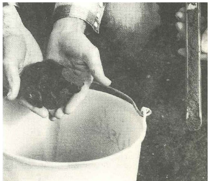
Figure 3. A soil probe takes uniform size cores and is a relatively easy tool to use when conditions in the soil or spoil permit.
