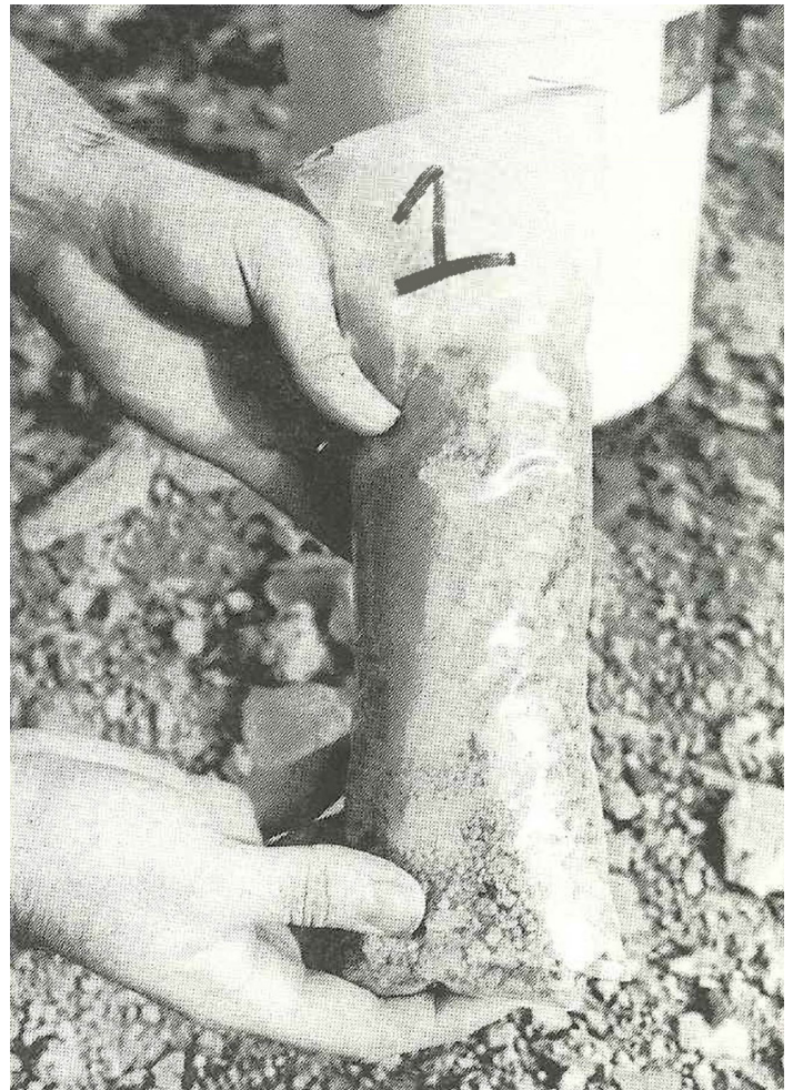
Figure 5. The mixed composite sample should be transferred from the bucket to a container, such as a plastic bag, and taken to the drying area.
