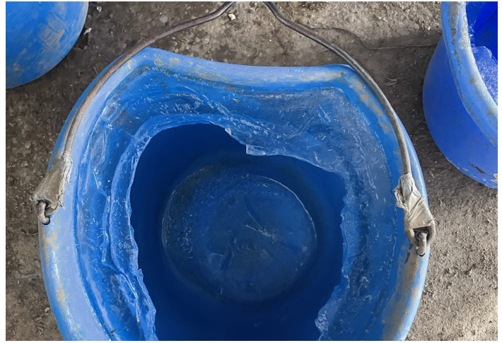
Figure 2. Duct tape wrapped around bucket handle ends.
