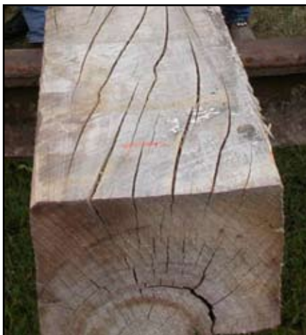
Figure 37. Since sweet gum normally has interlocking grain, the evident slope of grain in this tie would be acceptable. Figure 3 showed a good example of a sweet gum tie with interlocking grain, so it's repeated here. The shake would have to be looked at too.
