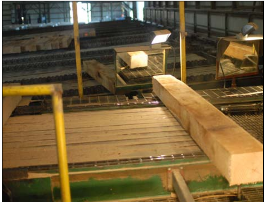
Figure 12. A hardwood tie as seen while being inspected by a tie grader. Notice the lights and mirrors aimed at the far end of the tie so the grader can look for holes and other defects.
