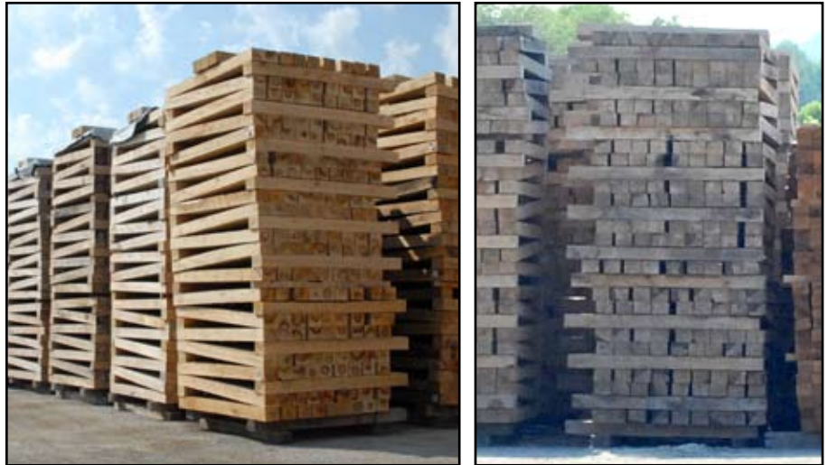
Figure 1. "German stacking," a common method of arranging ties for air drying in a tie yard. (The ties on the right could have been spread more uniformly for better air flow during drying, however.)
