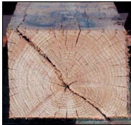
Figure 28. This tie could be saved with an end plate. Single "through splits" that equally divide the end are perfect for end-plating.
