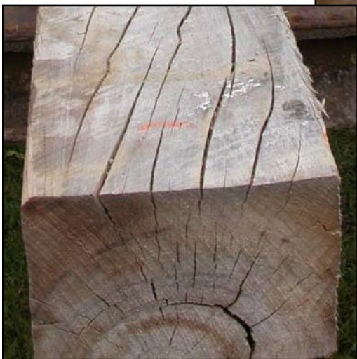
Figures 3 and 4. Compare the checking patterns on the sweet gum crosstie (above) to the white oak tie (right).
