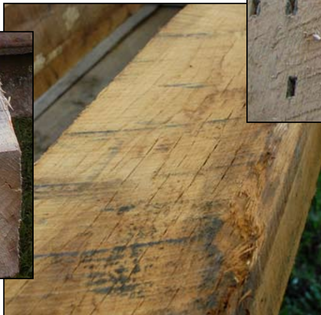
Figure 5. Mechanically incised tie.
