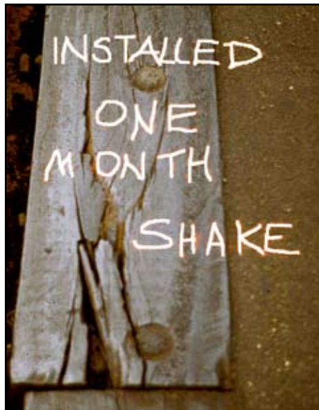
Figures 24 and 25. Early failures due to shake, one month old and one year old, respectively. The photo on the left is at a road crossing.
