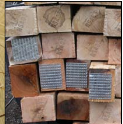
Figure 7. Some of these ties have been end-plated.
