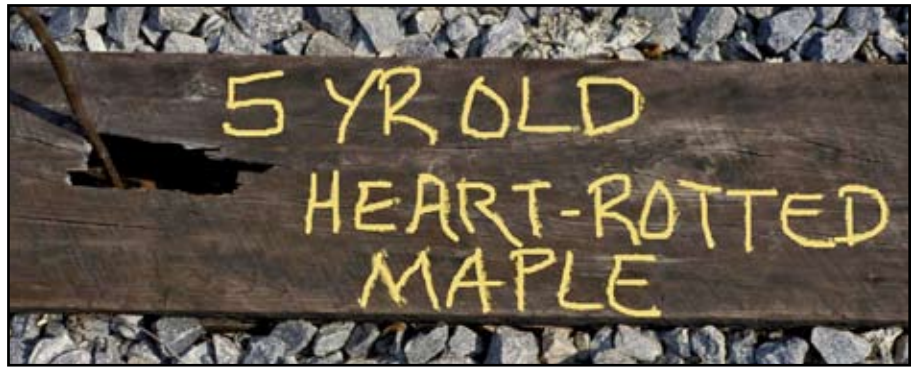
Figure 17. Heart-rotted maple tie after only five years in track.
