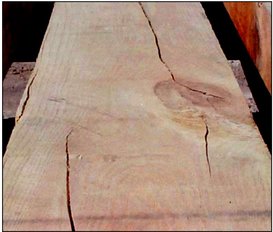
Figure 21. This large knot in the rail-bearing area is 3½" in diameter. Its size alone causes this tie to be culled, but notice that there is also some significant slope of grain associated with this knot. Even without the knot, the slope of grain would have to be examined as a potential reason to cull this tie.
