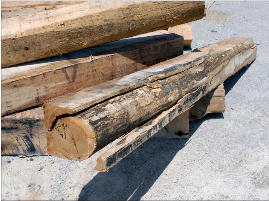
Figure 20. Shake can run the entire length of a log.
