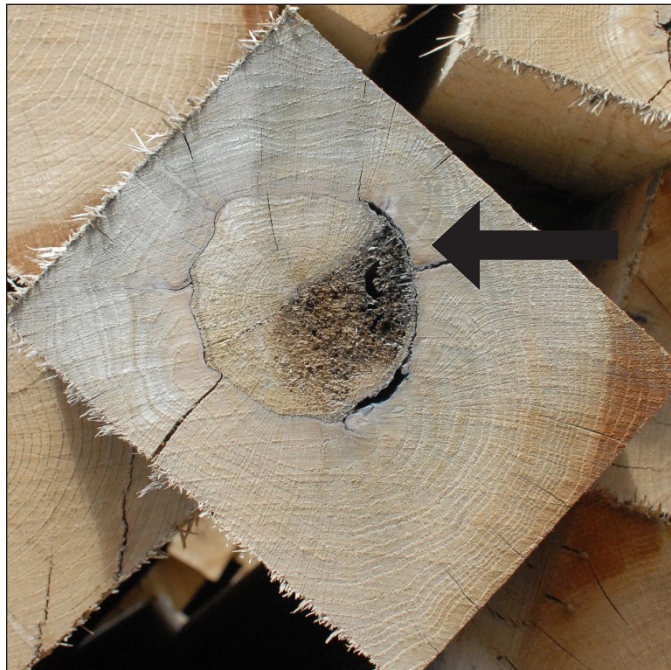
Figure 10. An oak tie showing fire scar with decay. (Arrow points to the tip of the fire scar).
