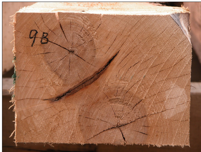
Figure 16. The bark seam in this twin heart hard maple doesn't look like it will extend very far, and therefore it would likely be acceptable.
