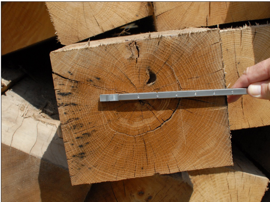
Figure 21. The shake in this 7" x 9" oak crosstie measures 4" across, making this an IG tie. If it were 3" wide or less it would have made a grade tie, because the shake doesn't appear to come to within 1" of any surface.
