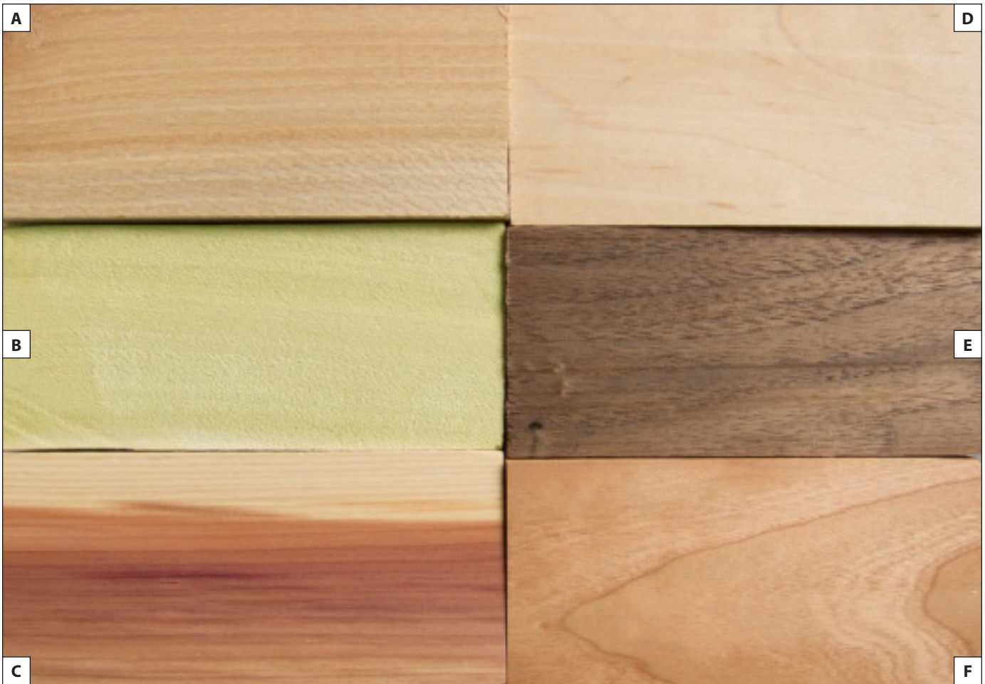
Figure 2-2. Examples of color variation in a few North American species: A: American sycamore, B: yellow-poplar, C: eastern redcedar (with sapwood), D: hard maple, E: black walnut, and F: black cherry. 4
