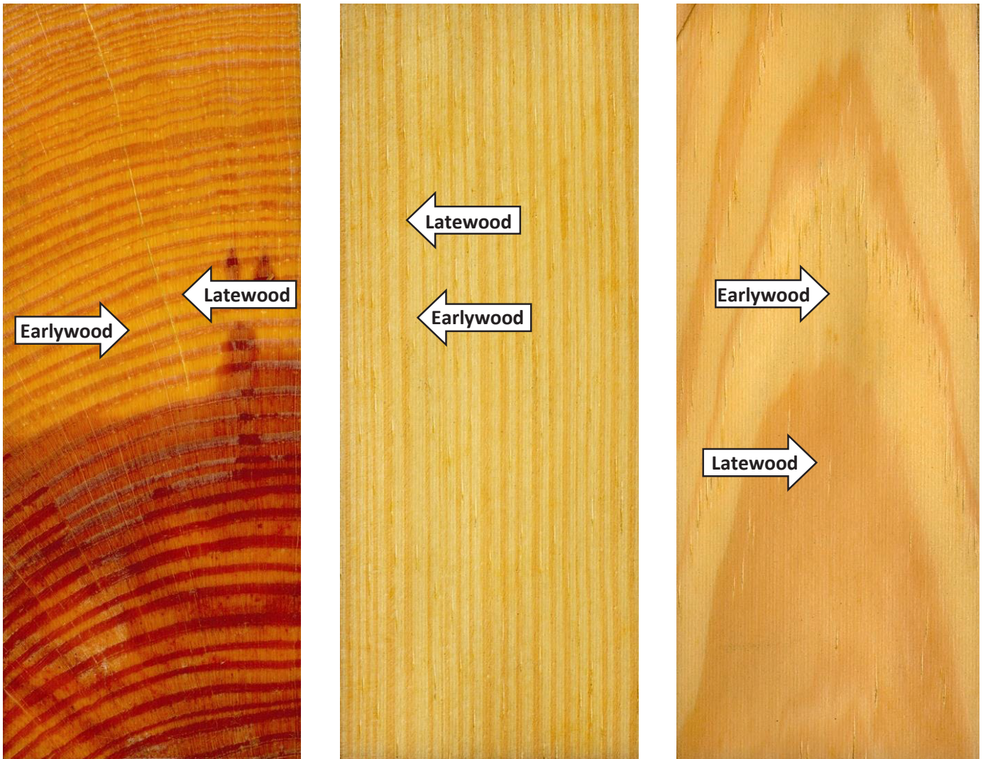
Figure 6-2. There is a clear distinction between the light-colored earlywood and the darker-colored latewood in each growth ring on these southern pine veneers (shown in x, r, t sequence). The abrupt transition between earlywood and latewood is easily visible on each plane. There are some streaks from resin canals visible on the tangential veneer photograph. These images are photographs of veneer sections from R.B. Hough's American Woods , shown actual size.
