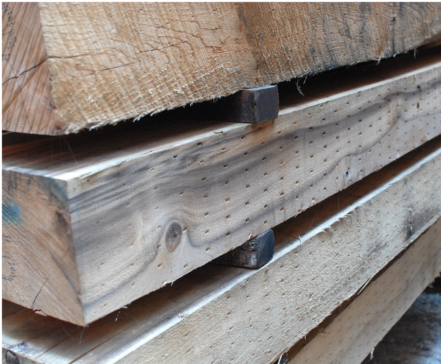
Figure 8-16. Another real-world example of growth ring differences between diffuse porous and ring porous species. In this photograph, a ring porous tie (red oak) is at the top and the central tie is diffuse porous (yellow-poplar). Notice the pulled fibers from the saw cut at the earlywood boundaries in the oak tie, and compare that to the smooth surface of the yellow-poplar tie. Notice the pulled fibers at the earlywood boundaries in the ring-porous tie, and compare that to the smooth surface of the diffuse porous tie. The regularly spaced marks are indentations (called incisions ) that are mechanically pressed into the ties to minimize long checks arising during shrinkage. Without incisions, some species tend to develop severe cracks, sometimes extending almost the entire length of the tie. Long checks are undesirable because they will degrade the mechanical performance of the ties.
