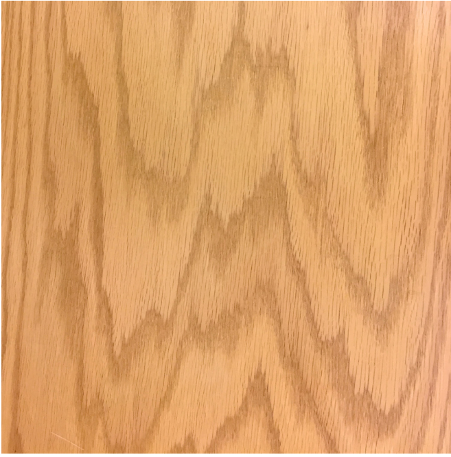
Figure 8-15. Photographs showing the differences between a ring porous hardwood (red oak, on the left) and a diffuse porous hardwood (hard maple, on the right). Note how the growth rings differ between the two species. In red oak, the earlywood pores are large and appear darker because they result in a greater effect of depth on the surface. In hard maple, the pores are not visible, and the growth rings are distinguished by the darker latewood fibers at the ends of the growth rings.
