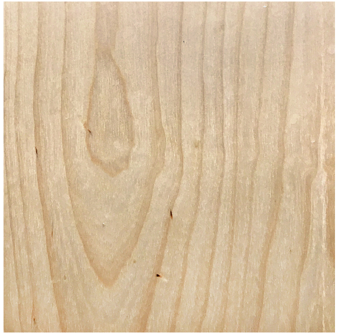
Figure 8-15. Photographs showing the differences between a ring porous hardwood (red oak, on the left) and a diffuse porous hardwood (hard maple, on the right). Note how the growth rings differ between the two species. In red oak, the earlywood pores are large and appear darker because they result in a greater effect of depth on the surface. In hard maple, the pores are not visible, and the growth rings are distinguished by the darker latewood fibers at the ends of the growth rings.
