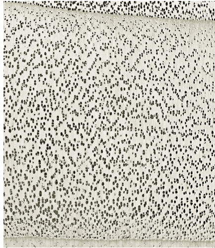
Figure 8-9. A micrograph of a piece of cottonwood ( Populus deltoides ) reproduced at a size that approximates the view you would see with a 10X hand lens. In this sample the pores all look about the same size for a large part of the growth ring, so this might be classified as diffuse porous even though the pores become noticeably smaller and sparser.
