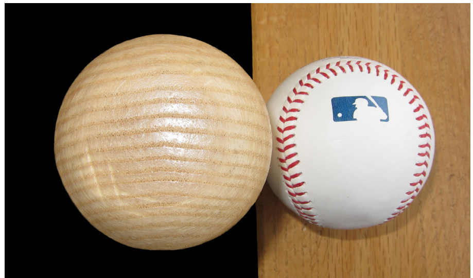
Figure 9-3. This illustration simulates what happens when a ballplayer hits a baseball on a radial surface with the edge of the growth rings pointed toward the ball. The baseball bat is made from a ring porous species, white ash ( Fraxinus americana ).
