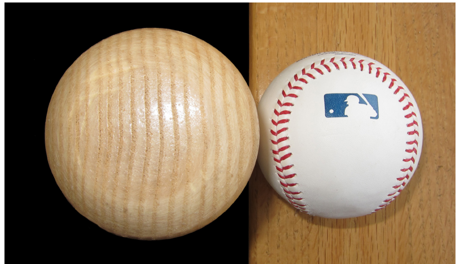
Figure 9-4. This illustration simulates what happens when a ballplayer hits a baseball on the tangential surface with the growth rings pointed straight up and down. This is the same piece of white ash ( Fraxinus americana ) used in the previous image.
