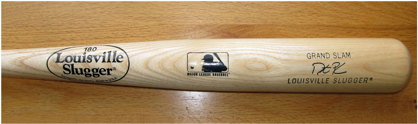
Figure 9-5. White ash baseball bat. The label is placed on the tangential face, so if the batter holds the bat with the label side up then the ball will strike a radial face (see Figure 9-1). The number 180 in the Louisville Slugger label on this bat means that this is a good quality amateur bat; the best bats (pro grade wood) are marked 125.
