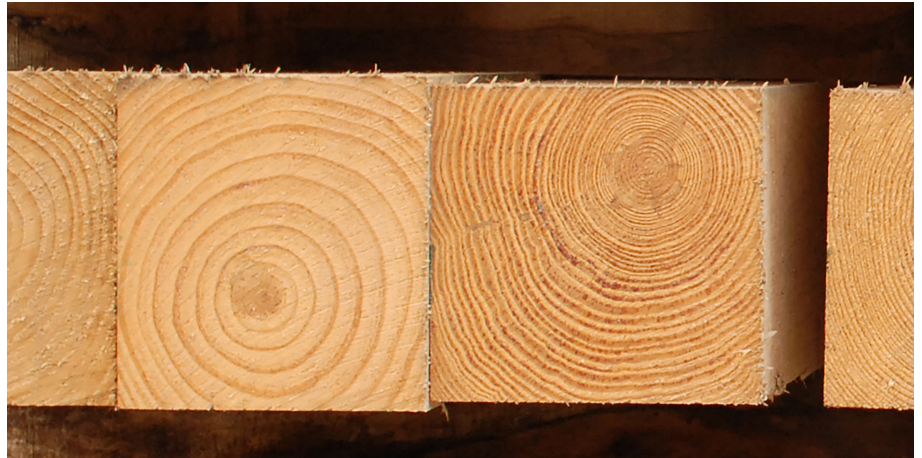
Figure 9-1. Two southern pine railroad ties. The tie on the left has wider growth rings and a lower percentage of higher density latewood compared to the slower-grown tie on the right.
