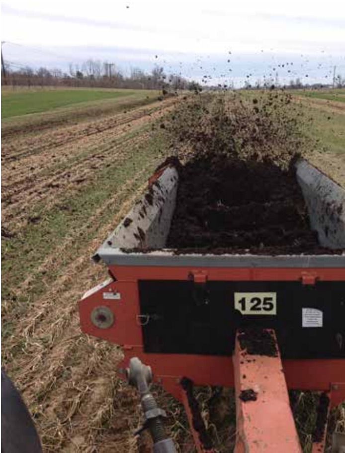
Figure 8. Spreading partially composted manure in fields with H&S PTO-driven manure spreader.
