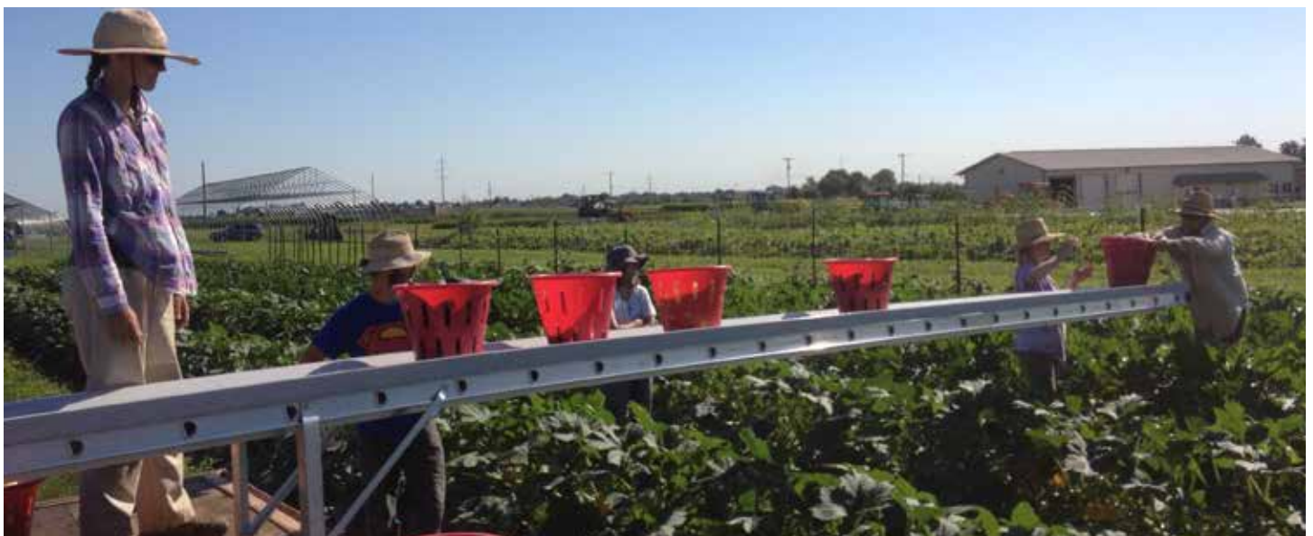
Figure 65. The harvest conveyor can carry filled buckets or individual crops.
