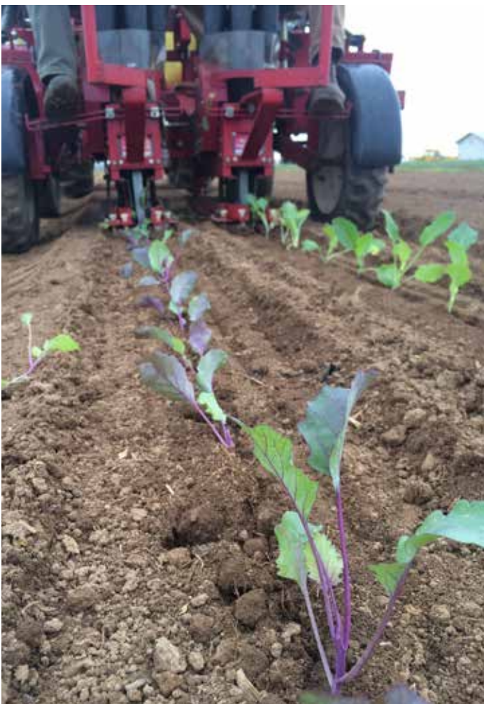
Transplanting with the Mechanical Transplanter planter.
