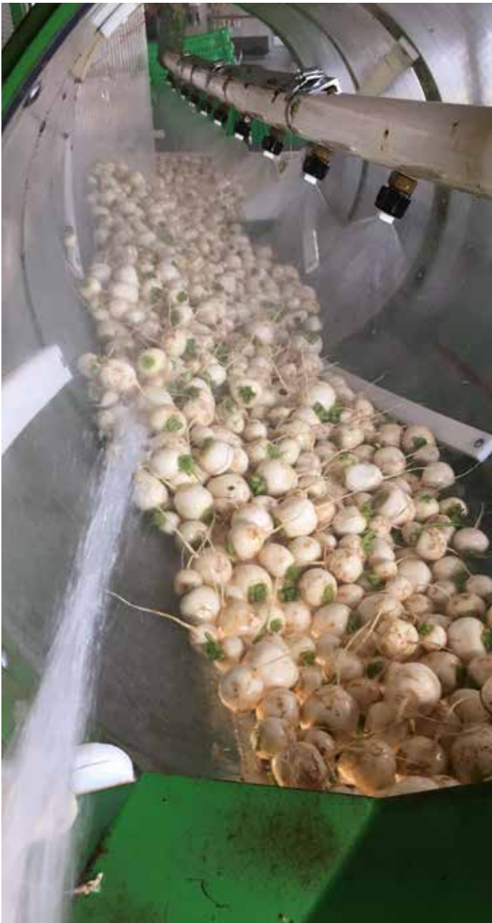
Loose roots are washed in the barrel washer, sorted, and weighed.
