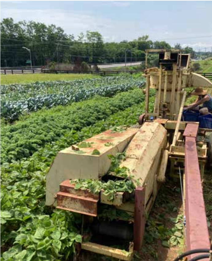
The Pixall BH100 Bean Harvester captures bean plants in a pair of tines that funnel plants into the picking reel.
