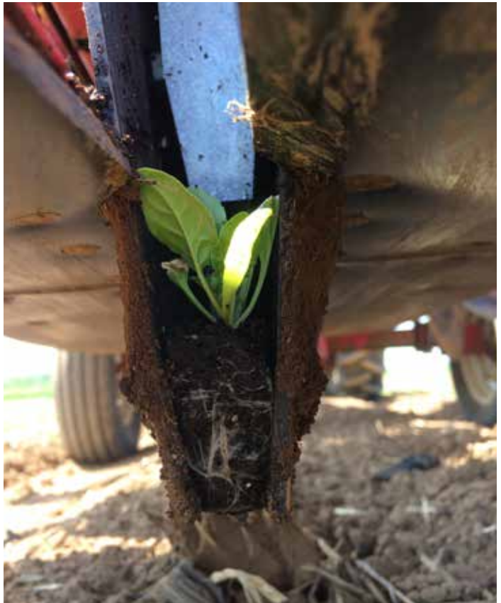
Figure 30. Plant plugs drop down chutes and get a spurt of water before being buried.
