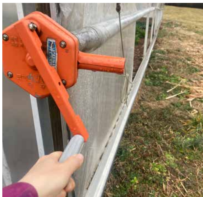
Figure 12.5 Winch to raise solar greenhouse curtain.
