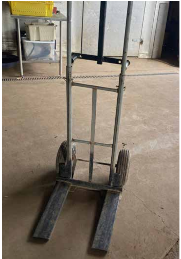
Figure 11.8 Custom hand truck with forks.
