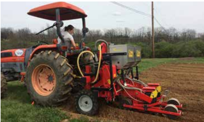
Figure 27. The MaterMacc VegiMacc vacuum seeder.
