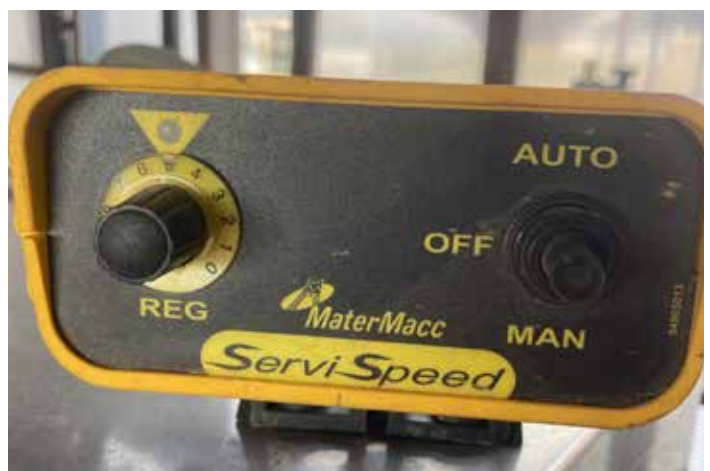
Figure 48. Control boxes are adjustable for fertilizer drop rate.
