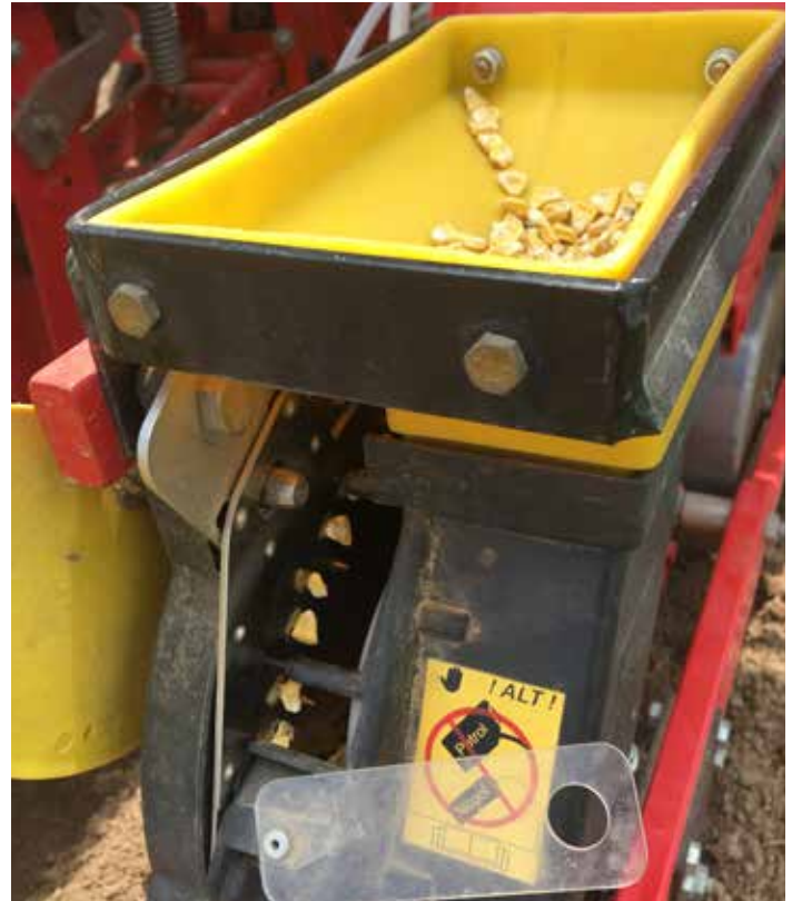
Corn is direct seeded with the MaterMacc VegiMacc.
