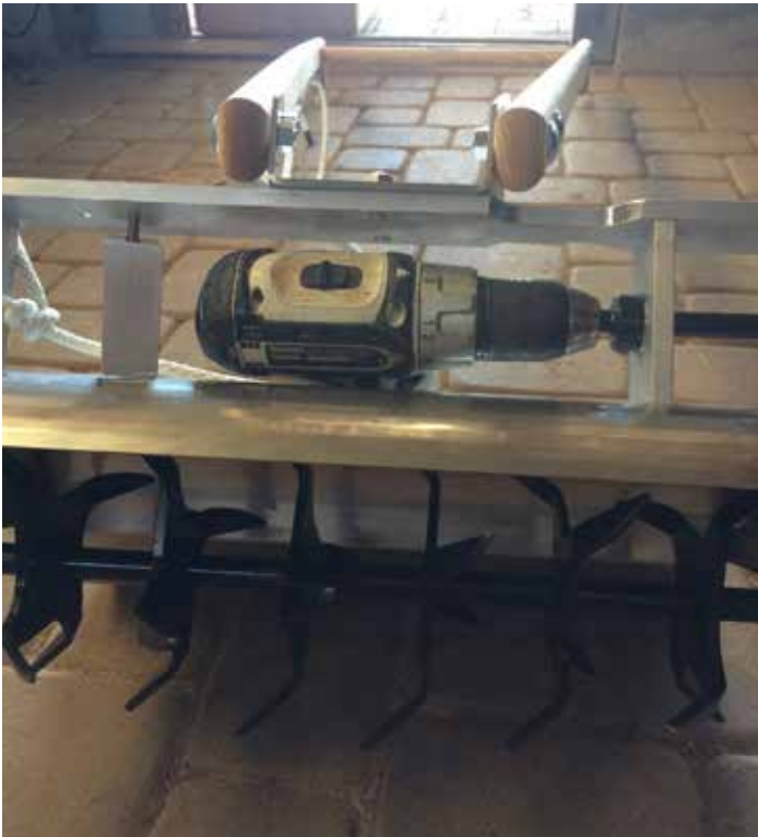
Figure 9. The Tilther, sold by Johnny's Selected Seeds, is run on a battery-powered drill. By pulling a rope connected to the drill, the tines are activated and rotate to incorporate compost, soil amendments, or small amounts of residue.
