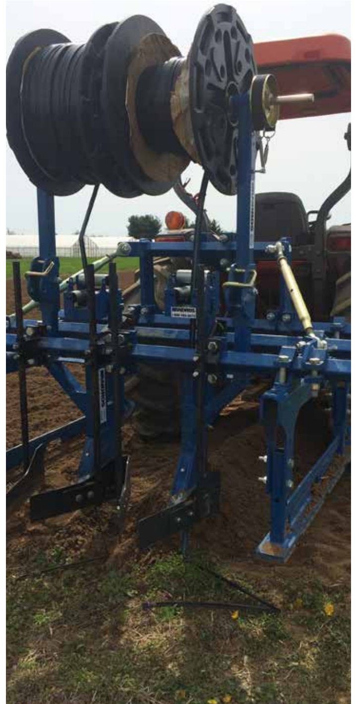
Figure 20. Custom Andros subsurface drip layer.
