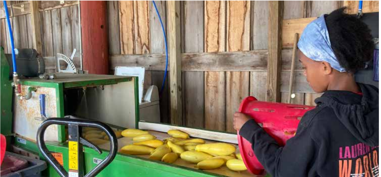
Squashes are loaded into the brush washer for washing, sorting, and packing.
