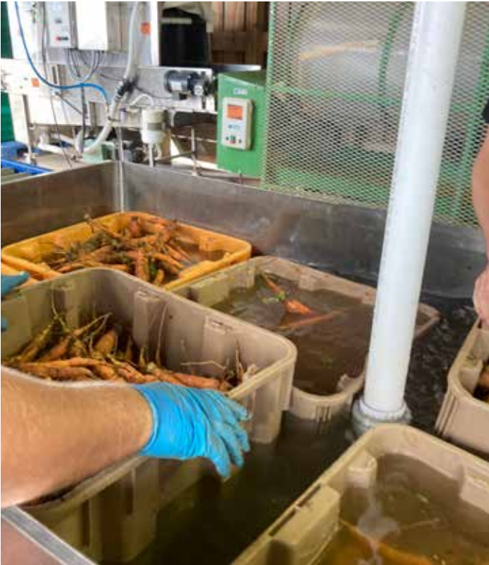
Six bins of carrots fit in dunk tank for bubbling.
