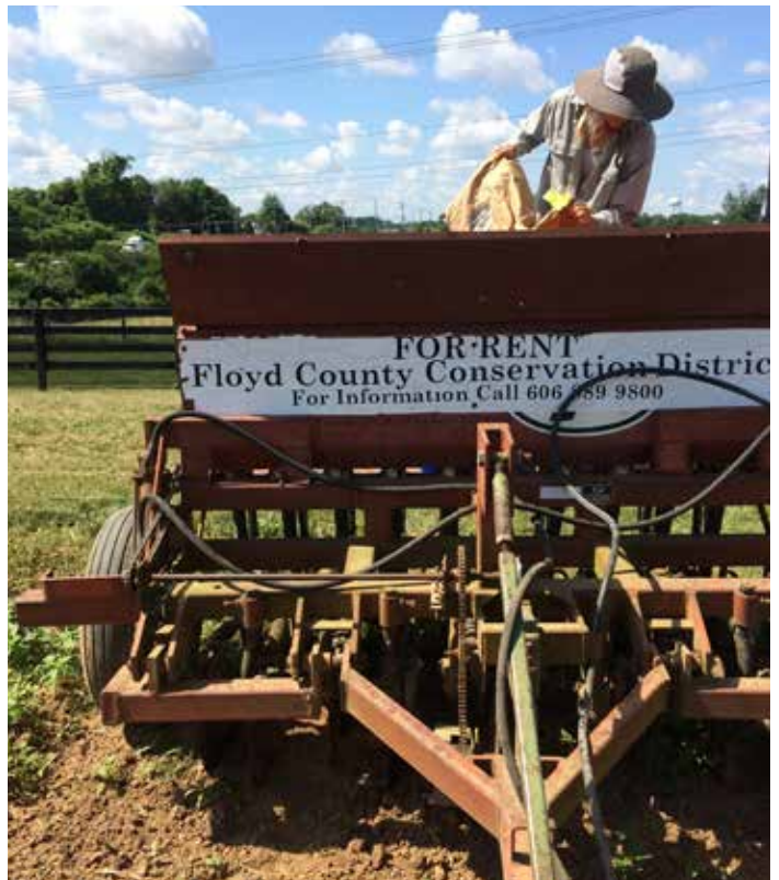
Figure 38. A worker fills the no-till grain drill with cover crop seed.
