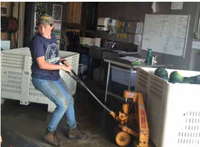
Figure 71. Pallet jacks maneuver macro bins and stacked pallets in the packing shed.
