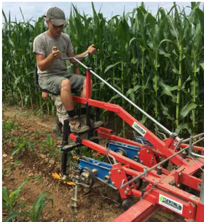
Figure 54. Kress Argus finger weeder.
