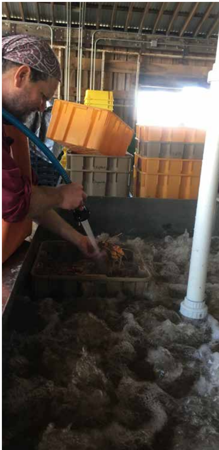
Turmeric is soaked in the dunk tank bubbler and sprayed off to remove soil.
