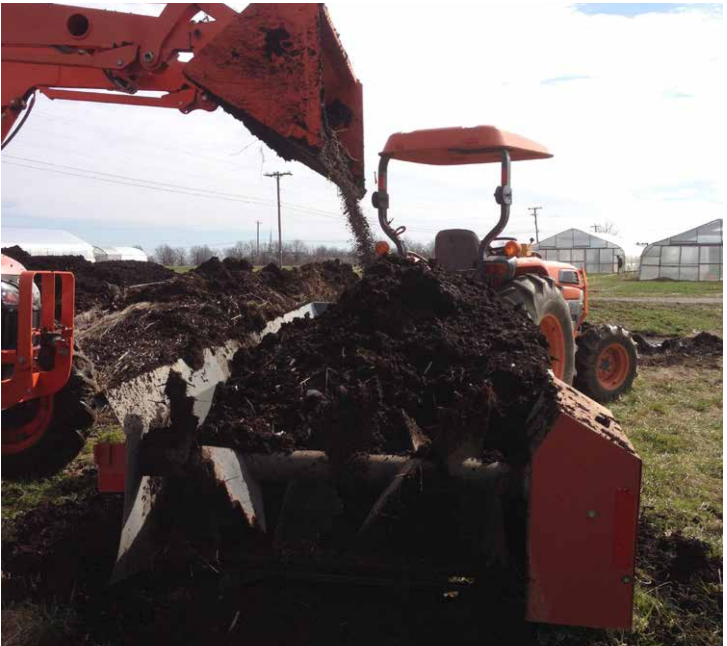
Figure 7. A bucket loader fills the manure spreader before it drives over the fields to spread the composted manure.
