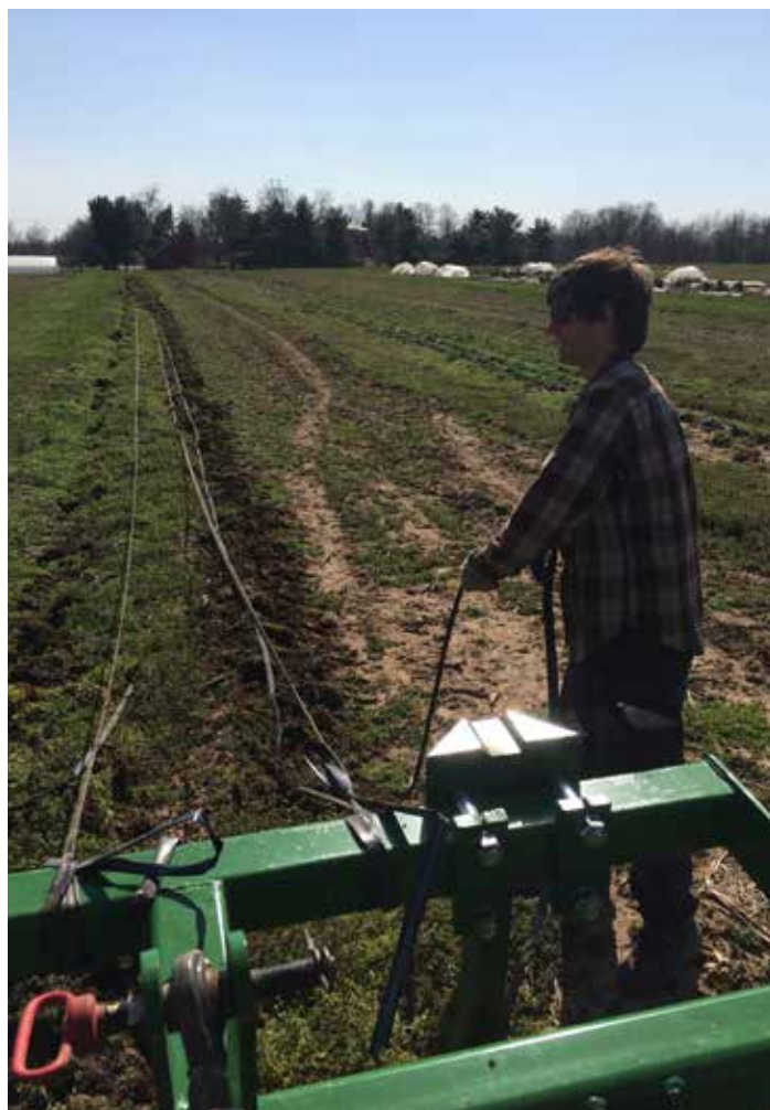
Figure 51. A drip lifter leaves the lines laying on top of the bed for easy pickup.
