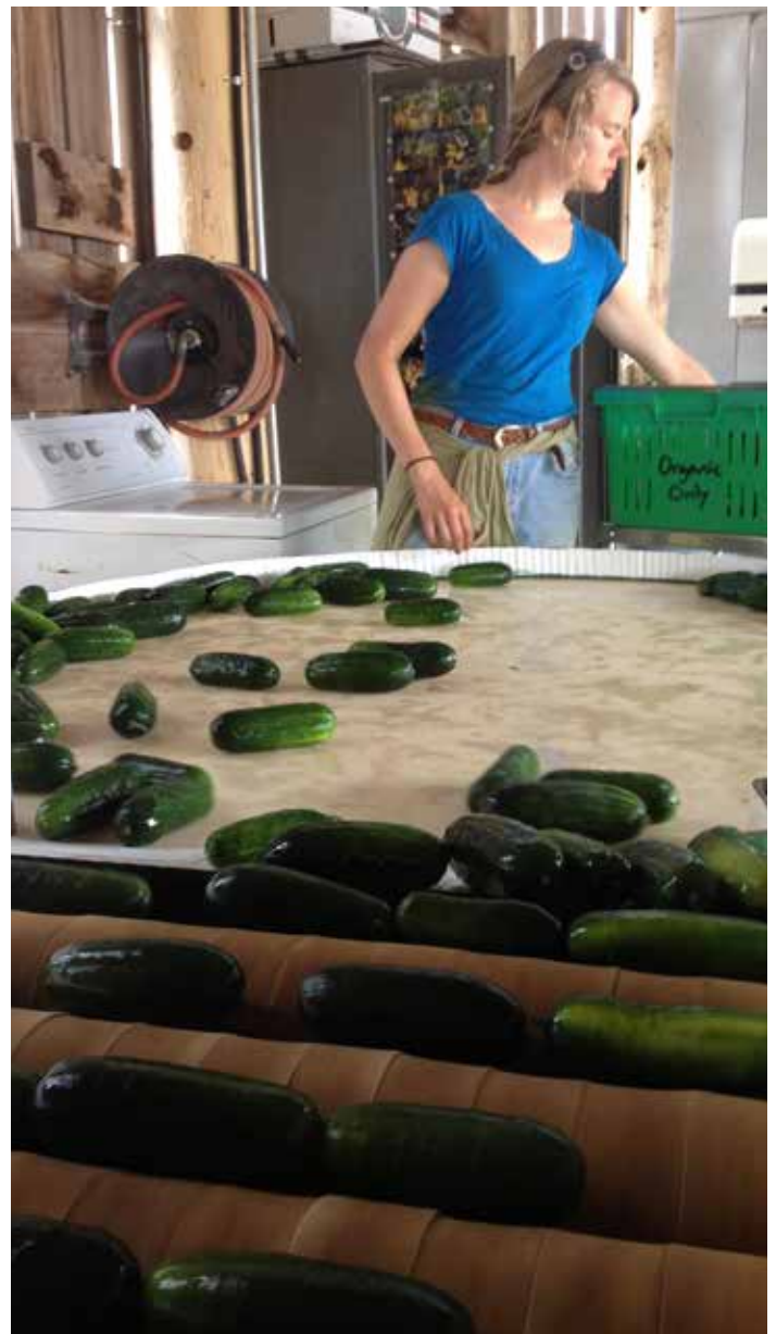
Cucumbers are washed on the brush washer and then counted into light-green bins.
