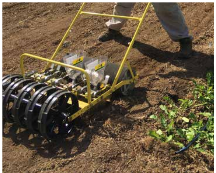
Figure 35. A six-hopper Jang push seeder can seed between one and six rows per bed at a time.
