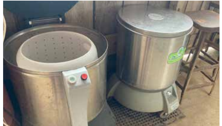
Two Electrolux industrial salad spinners work in tandem to remove excess water from leaves.
