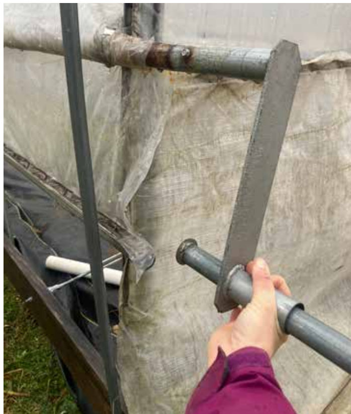
Figure 12.8 Handle crank on high tunnel side curtains.
