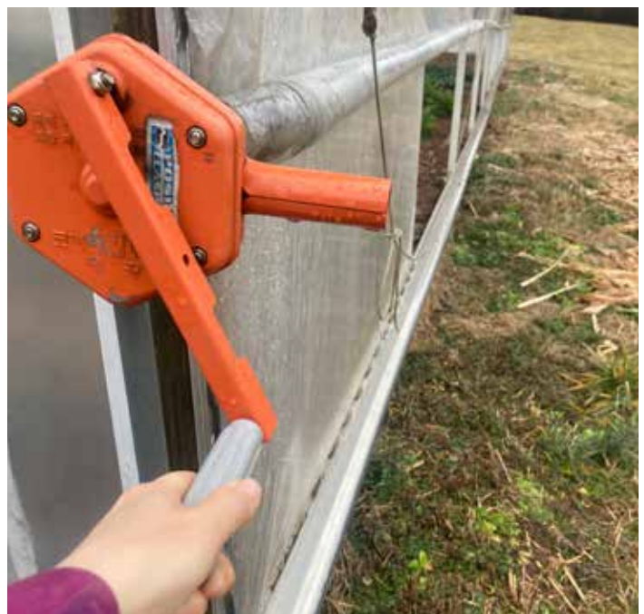
Figure 12.5 Winch to raise solar greenhouse curtain.
