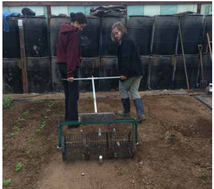
Figure 33. The 36-inch seedbed roller packs bed tops while dibbling holes. Dibble spacing is customizable.
