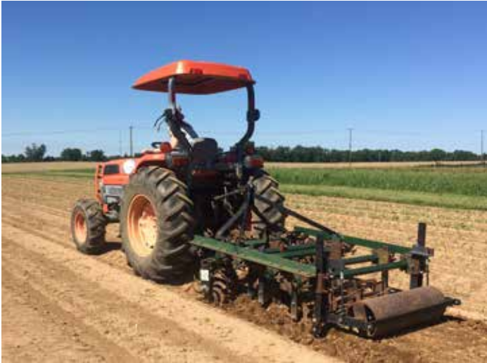
Figure 18. Custom stale seedbed cultivator.
