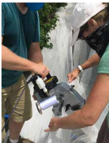
Two large pieces of ProtekNet netting are sewed together using a handheld sewing machine. Photo courtesy of Gonthier Lab.
