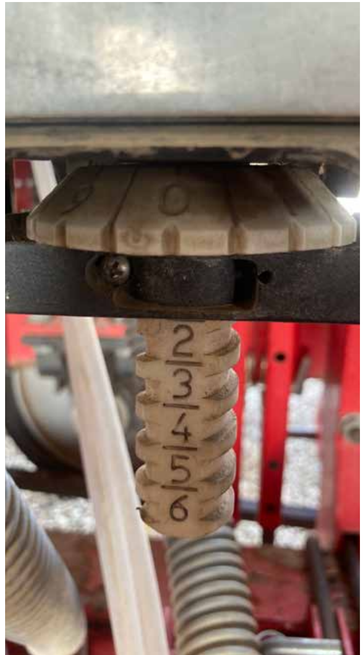
Figure 47. Fertilizer drop rate is adjusted by rotating the knob below the hopper.
