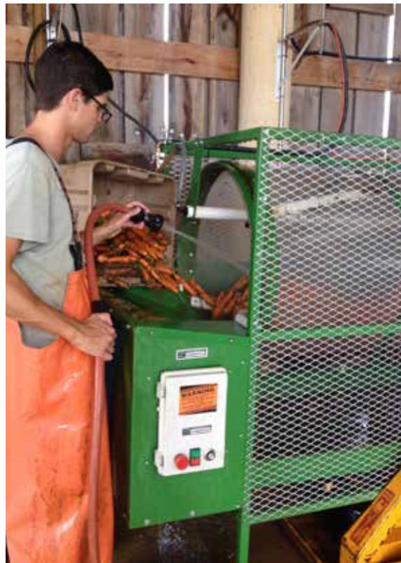
Loose carrots in barrel washer benefit from extra hose spray.
