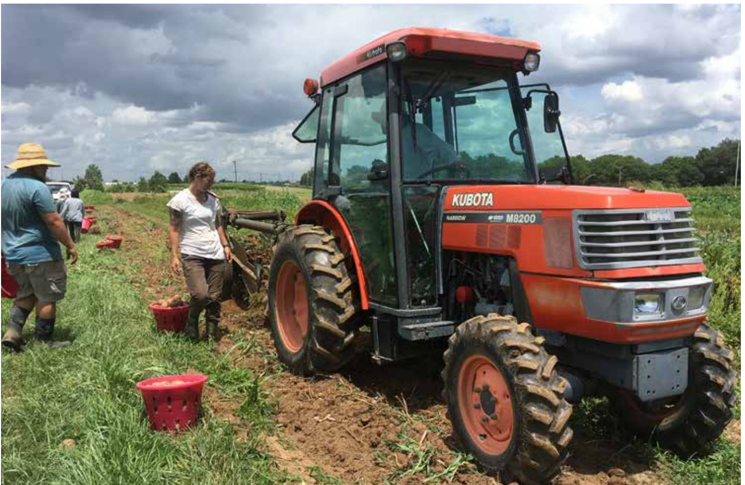
Potato harvest using the digger on the narrow Kubota M8200 tractor. Harvest buckets are spaced down the row.
