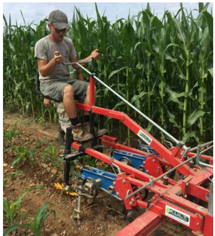
Corn is finger weeded when plants are four to eight inches tall.
