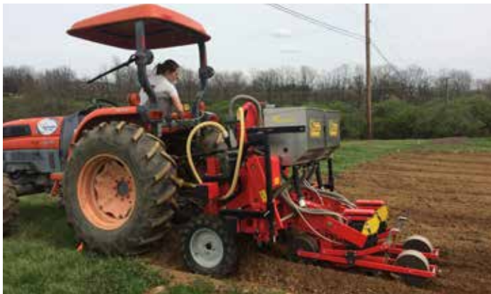
Figure 27. The MaterMacc VegiMacc vacuum seeder.
