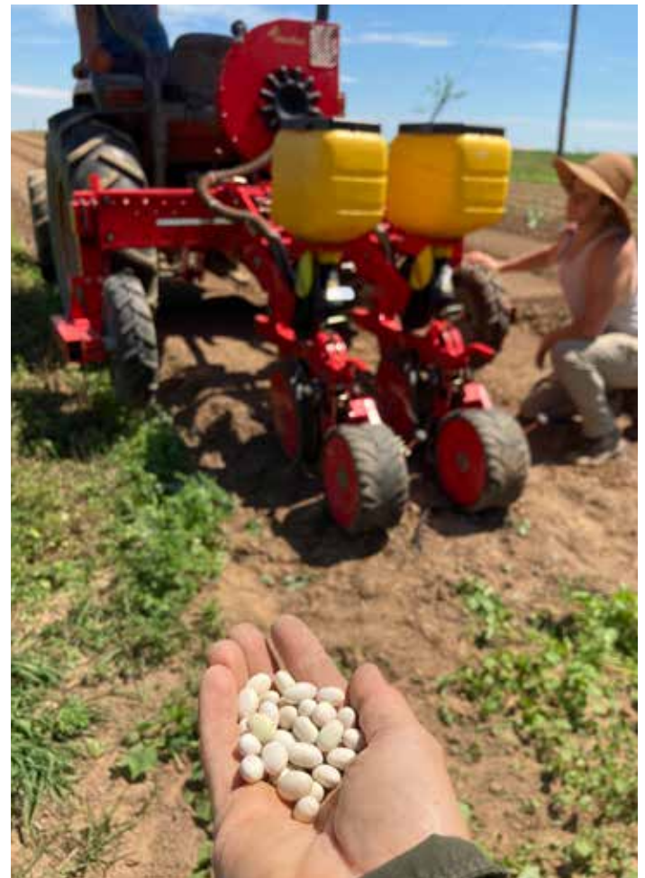
Beans are direct seeded with the larger of the two MaterMacc vacuum seeders.
