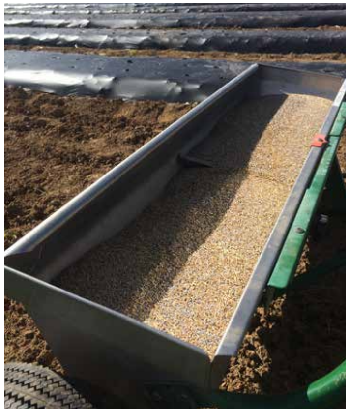
Figures 41 and 42. Drop spreaders suitable for undersowing and broadcasting living mulch seed between beds of plastic.
