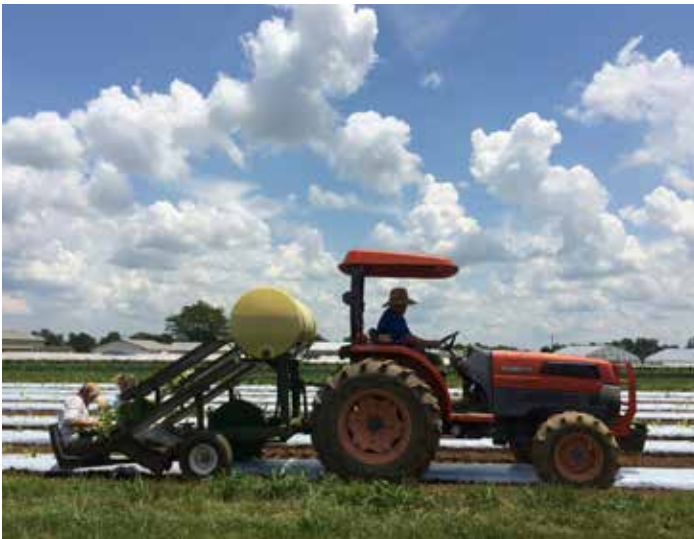
Figure 31. The Rain-Flo Model 1600 water wheel can hold one to three wheels for one- to three-row production systems. The wheel punches a hole into the plastic and creates a dibble, while a stream of water is sent into the hole.
