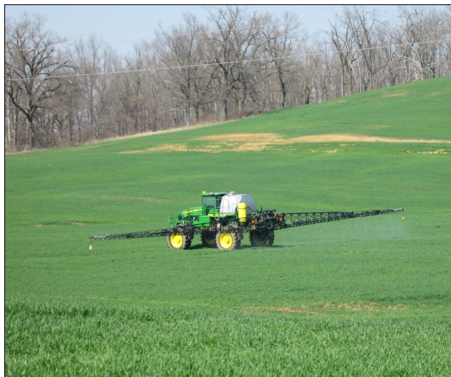
Photo 5-7. Most nitrogen fertilizer is applied as a liquid urea ammonium nitrate (UAN) and 28 or 32% N. By using stream bars or stream jet style nozzles, leaf burn from the UAN is minimized. Granular nitrogen (usually urea) can also be applied.
