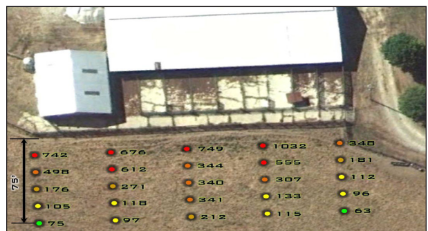
Figure 11. Soil test phosphorus concentrations adjacent to the partially-roofed backgrounding facility shown in Figure 10.
