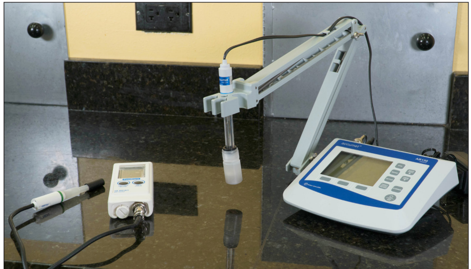
Figure 1. Two types of pH meters: the pen-like all-in-one unit (left), and the tabletop version (right).
