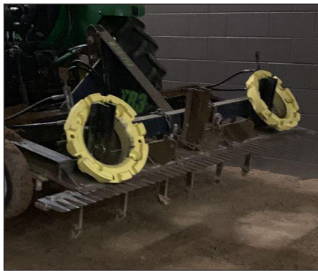
Figure 22. Sawtooth rake with weights.
