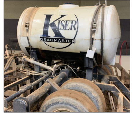
Figure 27. Water tank attached to drag.
