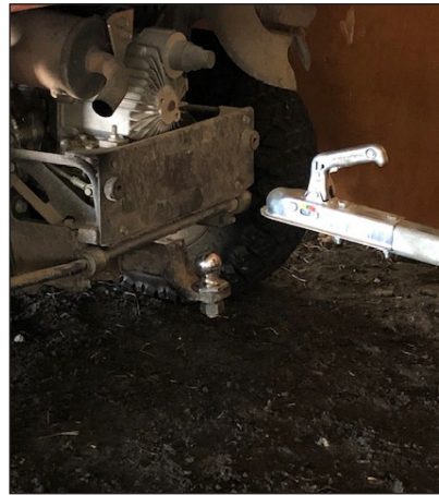
Figures 33 and 34. Ball hitch attachment method.
