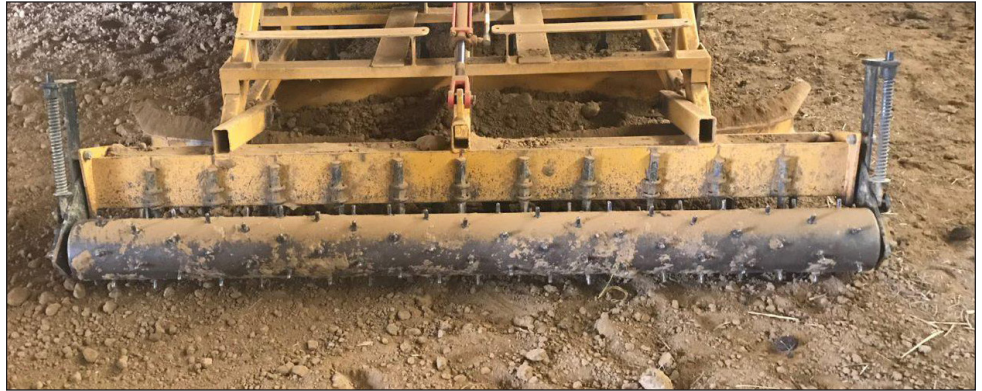
Figure 15. Sheepsfoot roller, part of a multi-unit drag.
