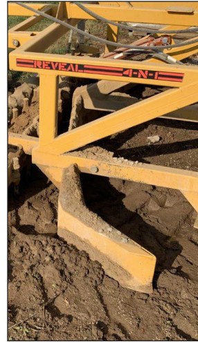
Figure 20. Box scraper, plated, part of multi-unit drag.
