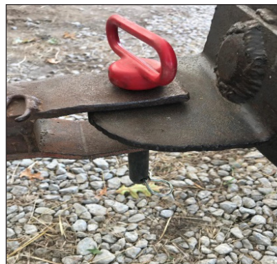
Figure 35. Draw bar attachment with hitch pin connection.
