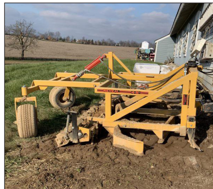
Figure 5. Hydraulically positioned drag.
