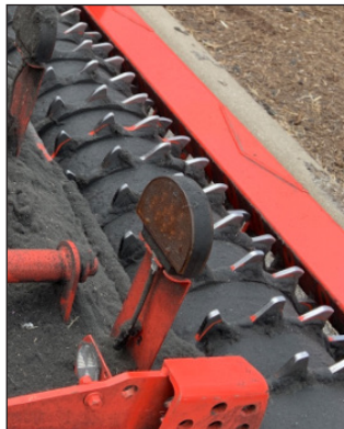
Figure 16. Sheepsfoot roller, part of a multi-unit drag.
