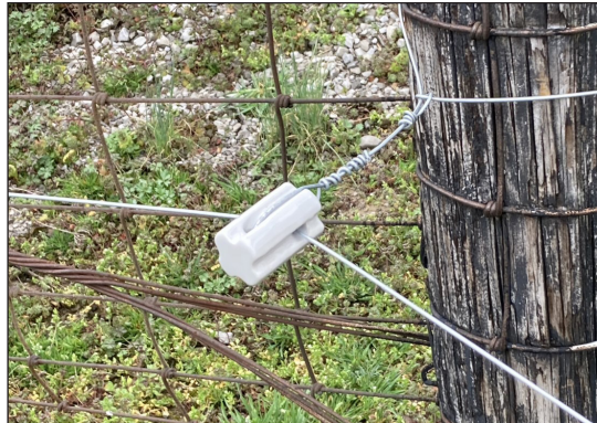
Figure 10. Doughnut or bullnose insulators can be used to make gentle bends in the offset that pull away from the post.
