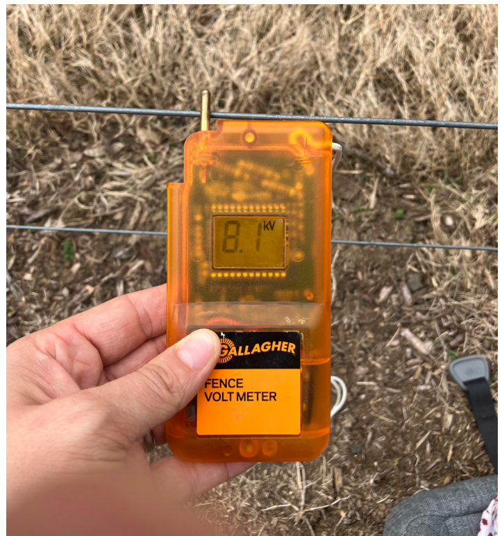
Figure 6. Voltmeters typically have a ground probe (white wire) that can be placed into the soil and a metal tip which can be placed onto an energized wire or port on the energizer. The output can be digital or analog, but both provide a reading in volts or kilovolts (1,000 volts) showing how 'hot' the fence is.
