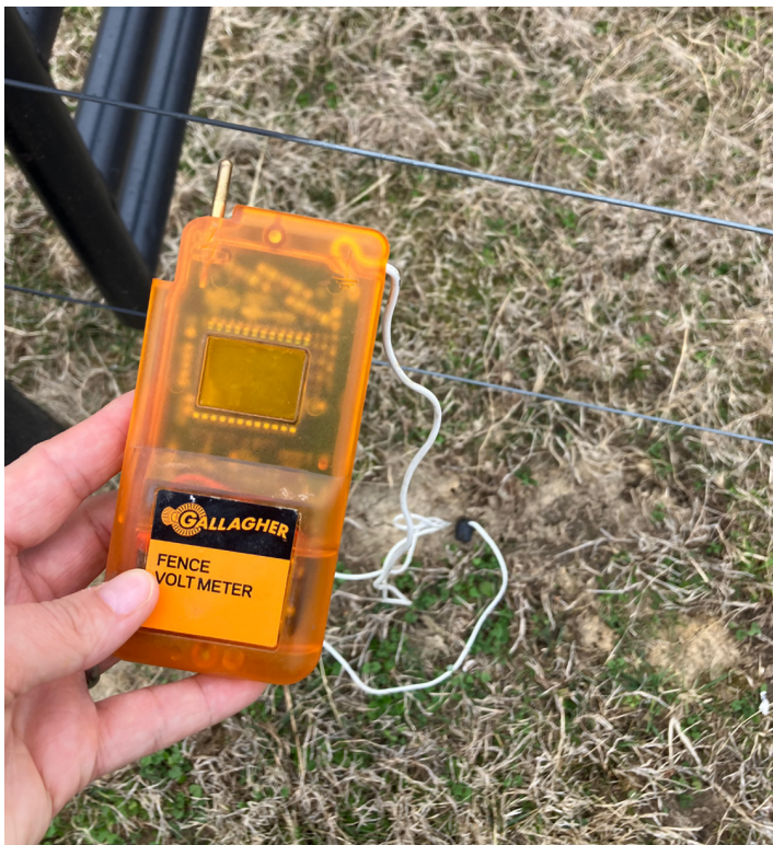
Figure 6. Voltmeters typically have a ground probe (white wire) that can be placed into the soil and a metal tip which can be placed onto an energized wire or port on the energizer. The output can be digital or analog, but both provide a reading in volts or kilovolts (1,000 volts) showing how 'hot' the fence is.
