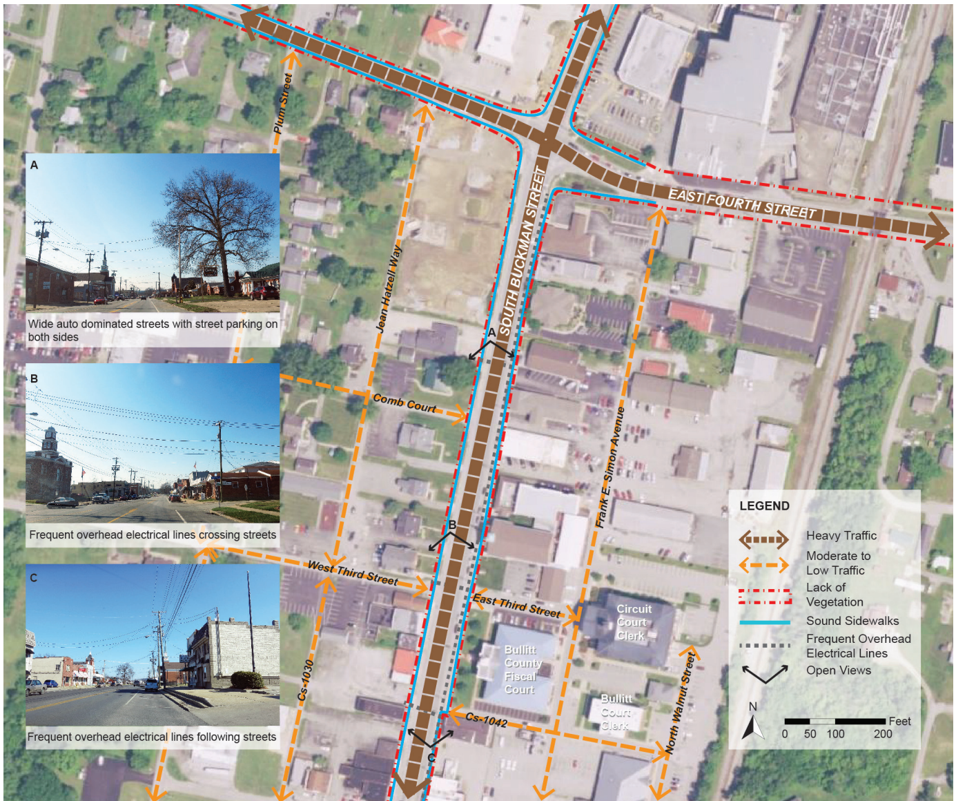
Figure 6. Context analysis map of South Buckman Street (US 61) and East 4th Street (US 44) in Shepherdsville, Kentucky Source: Basemap Imagery USDA FSA NAIP, 2017
