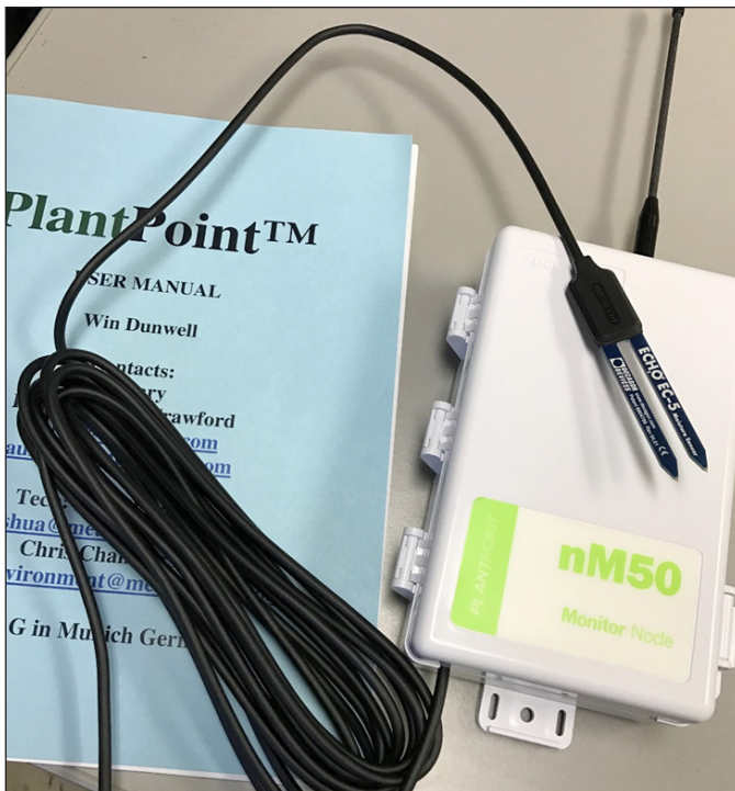
Figure 1. Echo-EC-5 moisture sensor, PlantPoint manual, nM50 wireless node.
