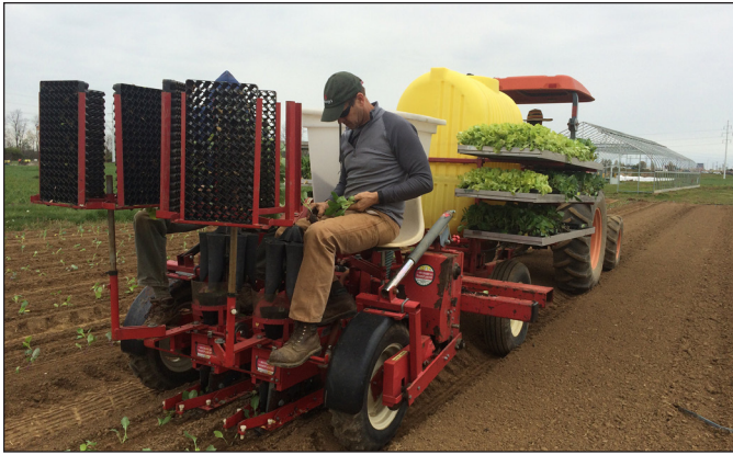
Figure 10. Mechanical Transplanter model 5000 with fertilizer hopper, water tank, and custom transplant tray holding racks.
