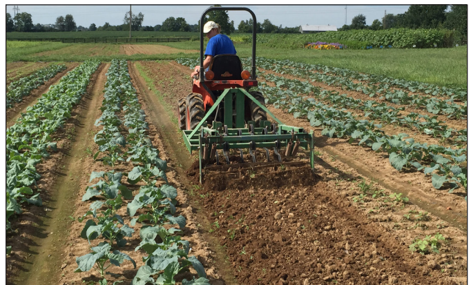
Figure 5. Kubota B1700 and custom 4 ft. field cultivator with a series of Danish S-tines and rolling basket.
