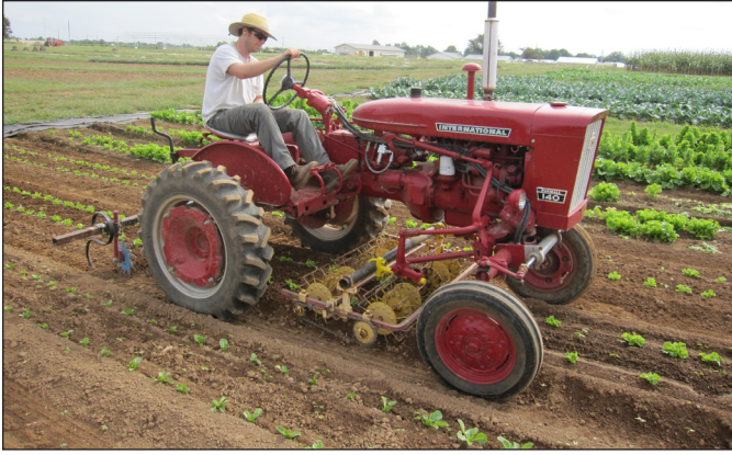
Figure 6. IH Farmall 140 with a custom power steering system, belly-mounted Buddingh basket weeders, and rear-mounted spyder and Danish S-tine cultivators.
