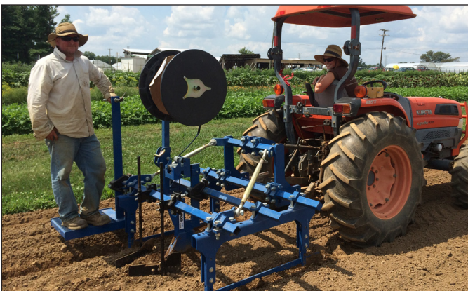
Figure 8. Custom Andros Engineering sub-surface drip irrigation layer.
