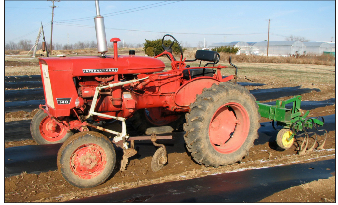
Figure 7. IH Farmall 140 with a custom power steering system, belly-mounted straight-tooth cultivators and small hilling discs for plastic bed-shoulder cultivation and rear-mounted Danish S-tines for wheel-track cultivation.
