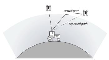
Figure 3. Atmospheric effects on radio signals.
