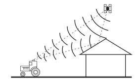
**Figure 4.** Multipath errors in GPS transmissions.
