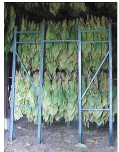
Figure 2. A two-tier pallet rack used in a tobacco barn driveway. (Note: diagonal bracing not visible.)
