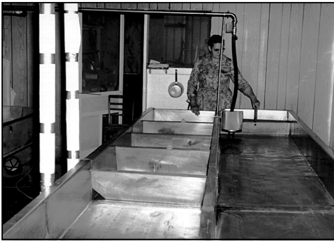
Figure 2. Shown above is a uniquely designed evaporation pan for large operations. The juice comes through the pan to the right, goes through a very fine wire strainer, and then up the pan to the left. Mrs. Donald Eck, Bartlett, Kansas, is holding the wooden skimming paddle.
