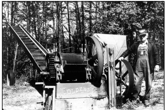
A typical large mill for squeezing the stalks
