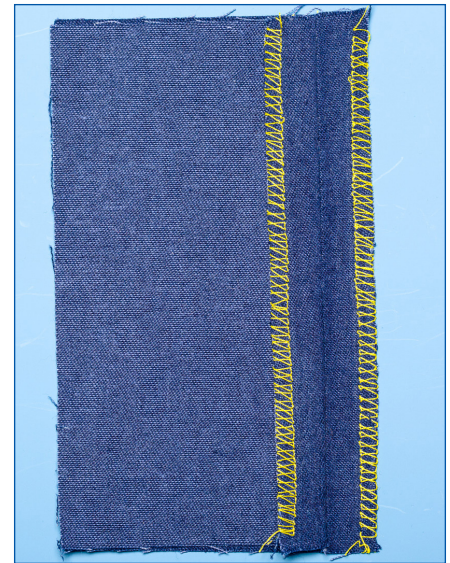
Machine overcast seam finish. Use the overcast presser foot.
