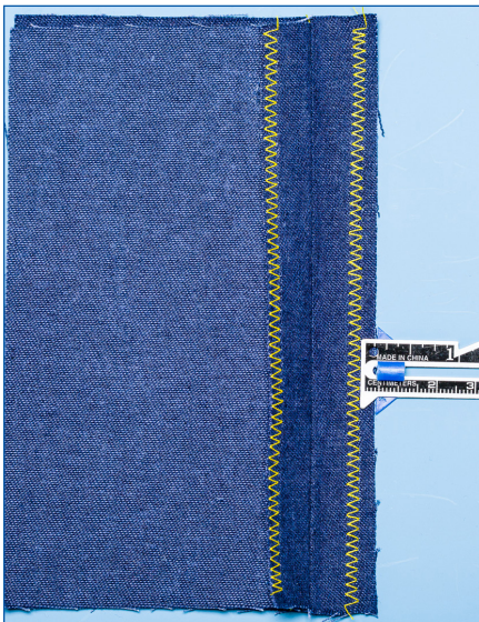
Zigzag seam finish. Zigzag 1/8 inch from raw edge; trim close to stitching.
