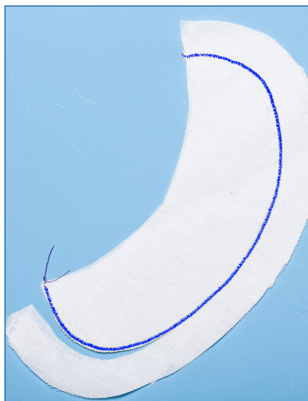
Hairline seam. Trim seam allowance close to zigzag stitching.
