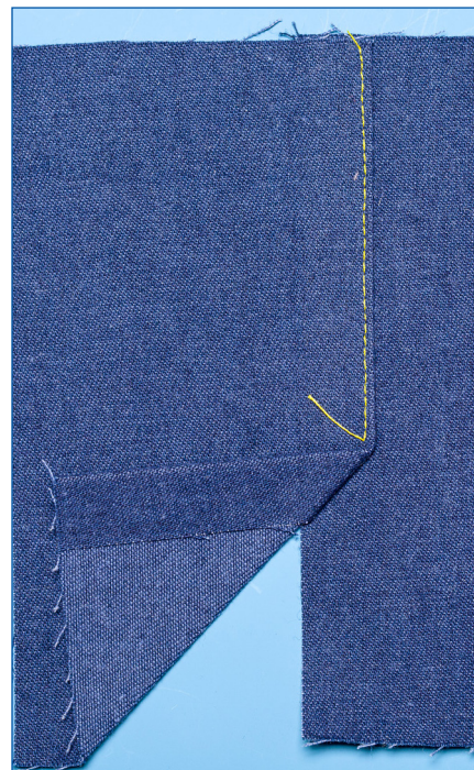
Lapped seam. Overlapping seam allowance on woven fabric is pressed under prior to top stitching.
