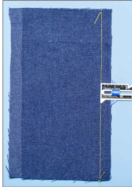
French seam. Sew the first line of stitching \frac{3}{8} inch from the edge.
