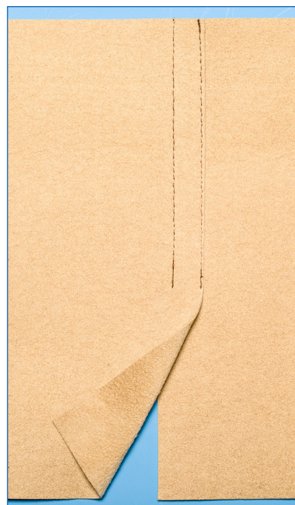
Lapped seam. Overlapping seam allowance on non-woven (Ultrasuede®) fabric is trimmed prior to top stitching.
