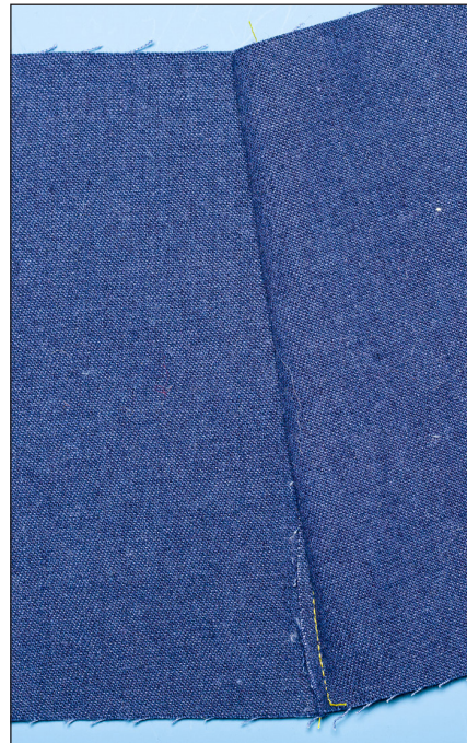
French seam. Raw edges of the trimmed seam allowance are enclosed within the seam.
