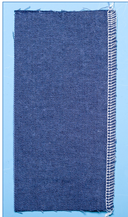
4-thread serged seam. Use for woven and knit fabrics that require stability.
