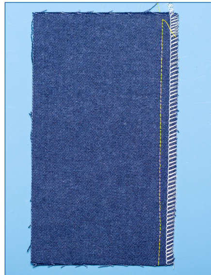
3-thread serged edge finish. Serge seam allowances together; press seam to one side.
