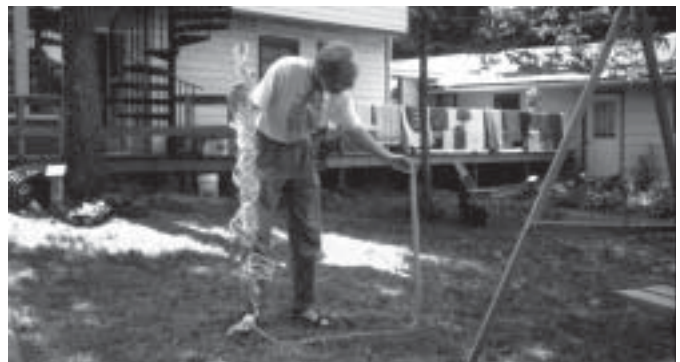
Figure 9. A water level with yardsticks on each end and the unused plastic tubing wrapped around one end.
