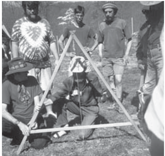
Figure 8. Using an A-frame with plumb line to find and follow contour lines.
