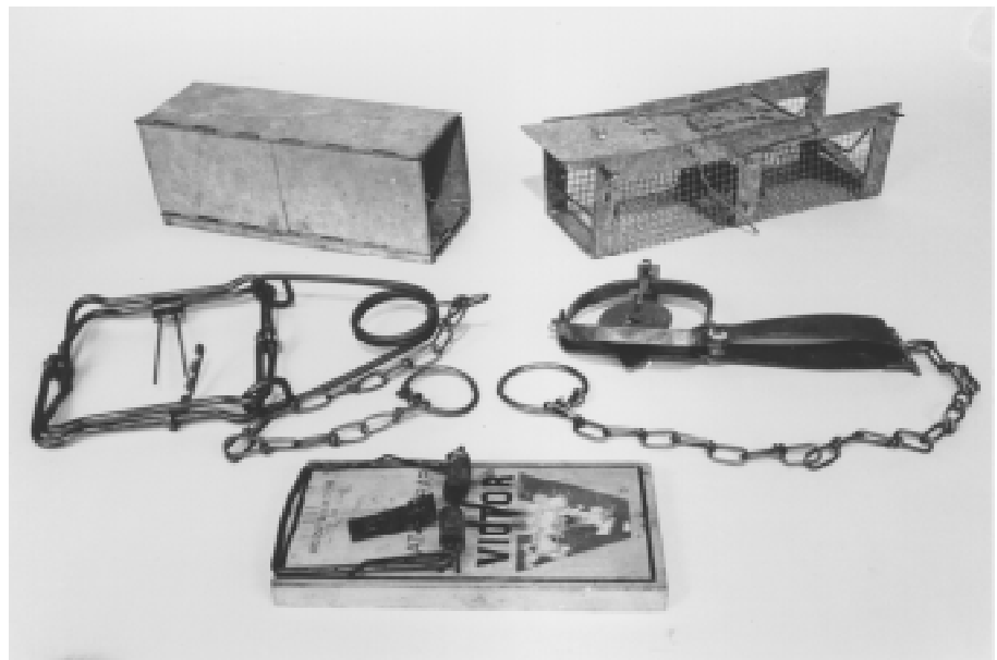
Figure 2. — Traps (clockwise from bottom): snap trap, Conibear trap, Sherman trap, cage trap, leg hold trap.
