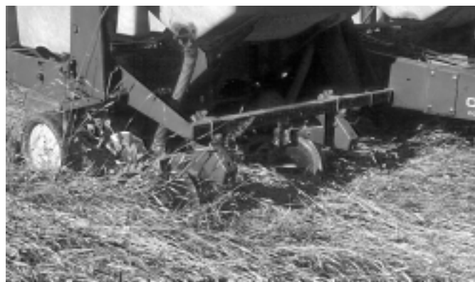
Figure 2. The no-till corn planter was modified for high surface residues: fluted coultter, residue cleaners in front of seeding unit, and spiked closing wheels, Berea, KY, 2002.
