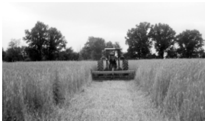
Figure 1. Rolling down the rye cover crop using a rolling stalk chopper before corn planting, Berea, KY, 2002.
